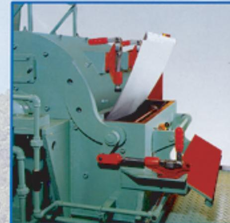
Rapid screen changer: Rapid and simple screen changing for the screen and need not to open its casing.
